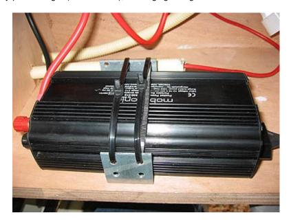
I did strap the unit into my 2<sup>nd</sup> battery box but you can also keep it separate if you don't want to fit it permanently to one vehicle only. This one uses two battery clamps but smaller once can be operated through the cigarette lighter.
