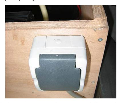
At the outside of my battery box you can find the 220 volt power point! The grey cable at the bottom will go to another power point in the back. I did use these waterproof ones because Land Rover will always leak!
