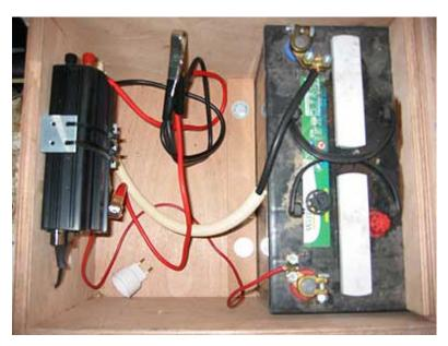
Here you can see the  $2^{nd}$  battery box in my vehicle (picture above). At the left hand side the 220volt inverter and at the right hand side the  $2^{nd}$  battery. Red thin cable is the charge one coming from the relay. The thick red & black ones with clamps can be clamped on the battery to operate the inverter get the 220volt. The thick black cable (partly covered in the protecting flexible hose) is the negative lead coming from the negative pole of the 1st battery.
