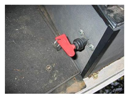
It's always wise to have a cut out switch for you battery and this one will disconnect both the batteries in one go from my vehicle.
