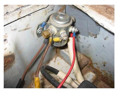
On the picture you can see the HD relay I am using. However the same can be done with a cheap plastic 30amp one which you can buy at every corner!
