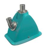
Our new Delta silencer/waterlocks are designed for use with Whisper generators positioned on or below the waterline. The Delta silencer systems have excellent acoustics, are high temperature proof and designed for any (Whisper) generator system from 3.5 to 20 kVA. The naval brass hose connections are suitable for 1%" or 2" ø hoses. Mounting bracket supplied as standard. Part # 50230093.
