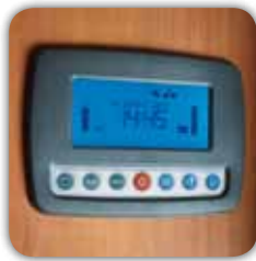
On board control panel (Toskana Exclusive)
